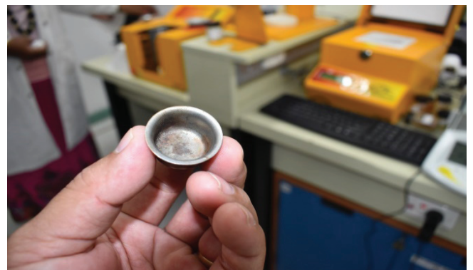
Figure 3: Shows Empty Crucible before filling with wood samples. (Peters et al, 2005)
