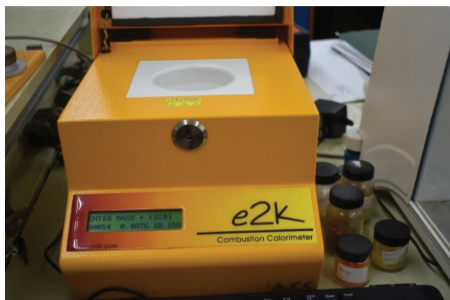
Figure 9: Shows the reading on the screen after combustion. (Peters et al, 2005)
