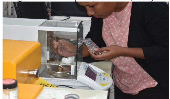
Figure 4: Shows a Forestry Research Staff weighing the wood samples in the crucible. (Peters et al, 2005)
