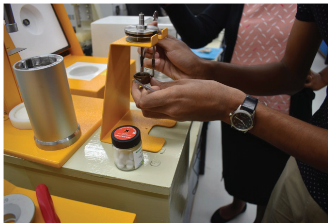
Figure 6: Shows the Forestry Research Staff burying the firing wire under the wood samples. (Peters et al, 2005)
