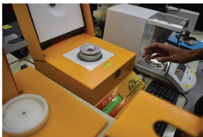
Figure 7: Shows the wood samples in the calorific tester. (Peters et al, 2005)
